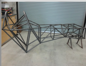
The chrome-moly steel frame for the car.
