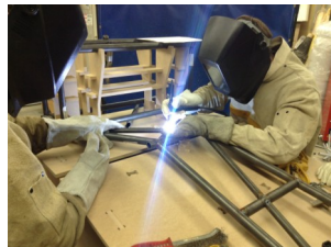
Daniel Woodside and Patrick McJannett weld the steel frame together
